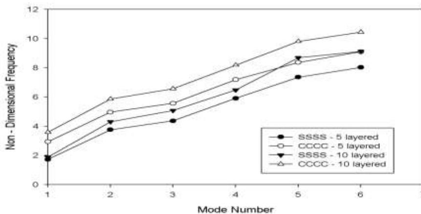
**Figure 5:** First six natural frequencies ( $\hat{\omega} = \left(\frac{\omega a^2}{\pi^2 h}\right) \sqrt{\rho/E_2}$ ) of symmetric five and ten layered cross ply ( $90^\circ/0^\circ/90^\circ\dots$ ),  $15^\circ$  skew laminated moderately thick ( $a/h=20$ ) plate ( $a/b=1$ ) with circular cutout for simply supported and clamped boundary conditions ( $K_s = 5/6$ ).
