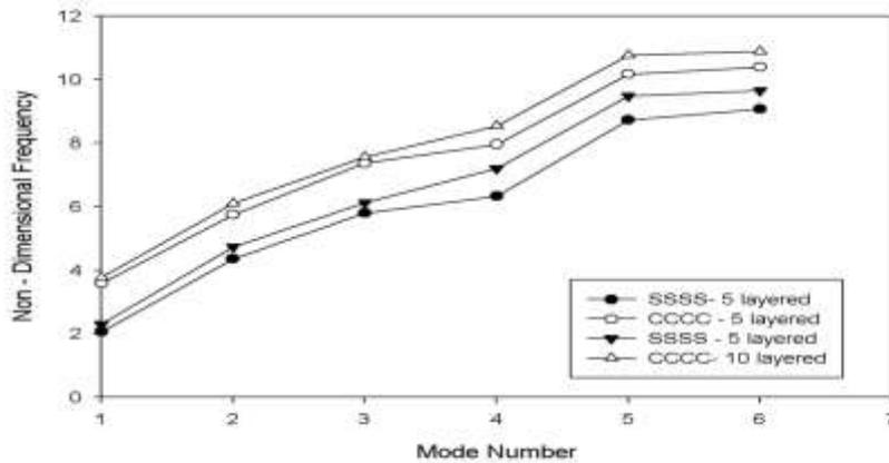
**Figure 10:** First six natural frequencies ( $\hat{\omega} = (\frac{\omega a^2}{\pi^2 h}) * \sqrt{(\rho/E2)}$ ) of symmetric five layered and ten layered angle-ply ( $-45^\circ/45^\circ/-45^\circ \dots$ ),  $30^\circ$  skew laminated thick ( $a/h=20$ ) plate ( $a/b=1$ ) with circular cutout for simply supported and clamped boundary conditions ( $K_s = 5/6$ ).
