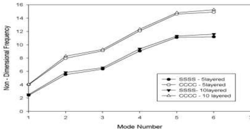
**Figure 4:** First six natural frequencies ( $\hat{\omega} = \left(\frac{\omega a^2}{\pi^2 h}\right) \sqrt{\rho/E_2}$ ) of symmetric five and ten layered angle-ply ( $-45^\circ/45^\circ/-45^\circ\dots$ ),  $15^\circ$  skew laminated thin ( $a/h=1000$ ) plate ( $a/b=1$ ) with circular cutout for simply supported and clamped boundary conditions ( $K_s = 5/6$ ).
