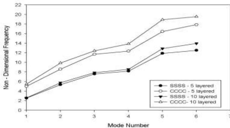
**Figure 7:** First six natural frequencies ( $\hat{\omega} = \left(\frac{\omega a^2}{\pi^2 h}\right) \sqrt{\rho/E2}$ ) of symmetric five layered and ten layered cross ply (90°/0°/90°...), 30° skew laminated thin (a/h=1000) plate (a/b=1) with circular cutout for simply supported and clamped boundary conditions ( $K_s = 5/6$ ).
