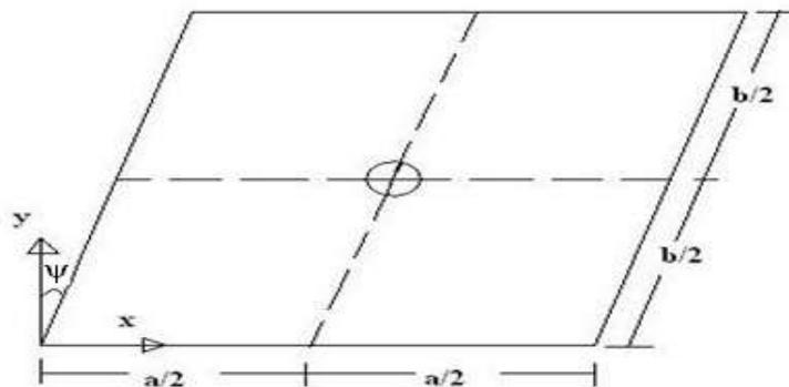
**Figure 1:** Skew laminated plate with circular cutout
