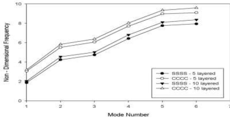
**Figure 6:** First six natural frequencies ( $\hat{\omega} = \left(\frac{\omega a^2}{\pi^2 h}\right) \sqrt{\rho/E2}$ ) of symmetric five and ten layered angle-ply (-45°/45°/-45°...), 15° skew laminated moderately thick (a/h=20) plate (a/b=1) with circular cutout for simply supported and clamped boundary conditions ( $K_s = 5/6$ ).
