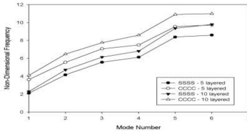
**Figure 9:** First six natural frequencies ( $\hat{\omega} = (\frac{\omega a^2}{\pi^2 h}) * \sqrt{(\rho/E2)}$ ) of symmetric five layered and ten layered angle-ply ( $90^\circ/0^\circ/90^\circ \dots$ ),  $30^\circ$  skew laminated thick ( $a/h=20$ ) plate ( $a/b=1$ ) with circular cutout for simply supported and clamped boundary conditions ( $K_s = 5/6$ ).
