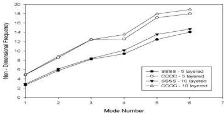
**Figure 8:** First six natural frequencies ( $\hat{\omega} = \left(\frac{\omega a^2}{\pi^2 h}\right) \sqrt{\rho/E2}$ ) of symmetric five layered and ten layered angle-ply (-45°/45°/-45°...), 30° skew laminated thin (a/h=1000) plate (a/b=1) with circular cutout for simply supported and clamped boundary conditions ( $K_s = 5/6$ ).
