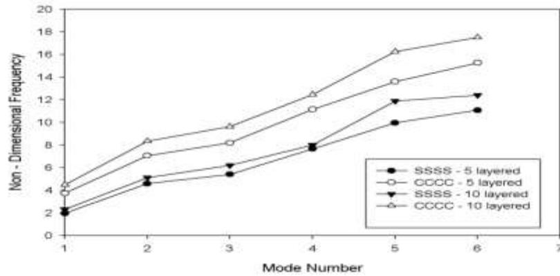
**Figure 3:** First six natural frequencies ( $\hat{\omega} = \left(\frac{\omega a^2}{\pi^2 h}\right) \sqrt{\rho/E_2}$ ) of symmetric five and ten layered cross ply ( $90^\circ/0^\circ/90^\circ\dots$ ),  $15^\circ$  skew laminated thin ( $a/h=1000$ ) plate ( $a/b=1$ ) with circular cutout for simply supported and clamped boundary conditions ( $K_s = 5/6$ ).
