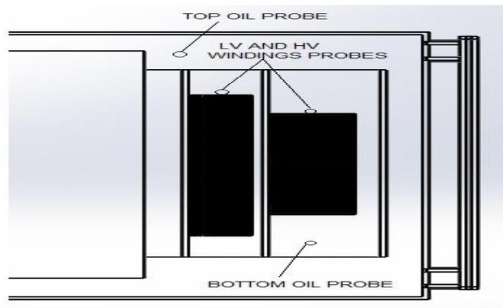
Figure 4b Location of probes in the power transformer
