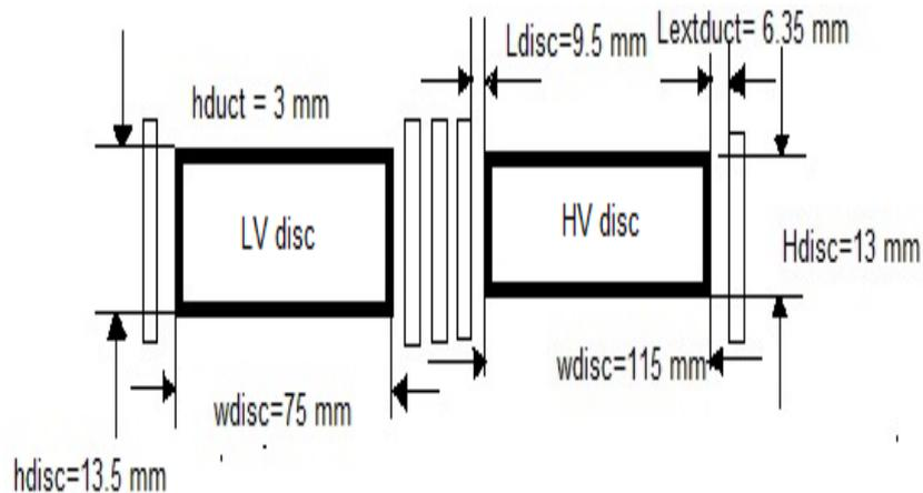
Figure 4 Dimensions of discs and cooling ducts
