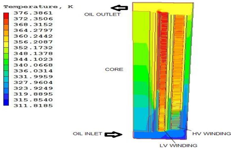
**Figure 5** Temperature contour (basic case: 82 and 102 discs for the HV and LV windings)
