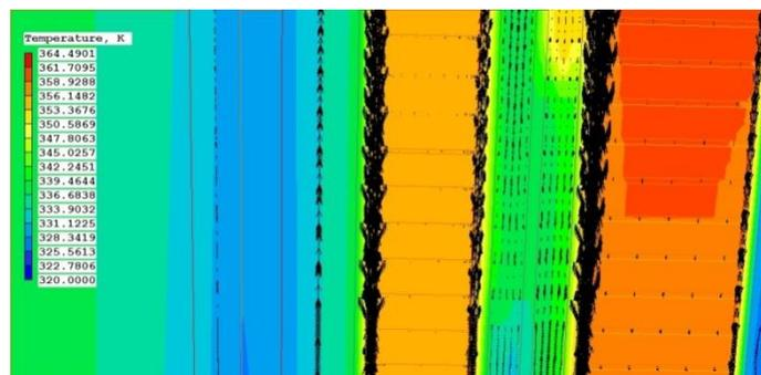
Figure 18 Closeup of winding temperature for the 4 mm HV duct width
