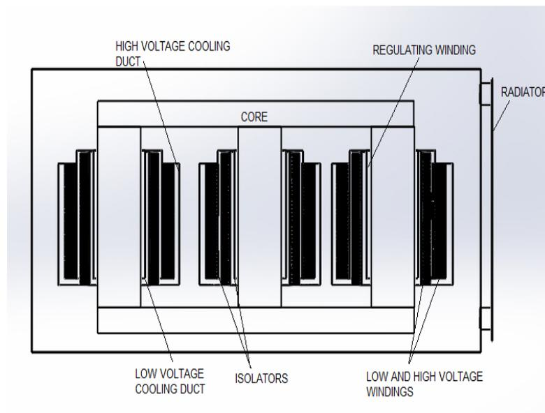
**Figure 1** Geometry of the transformer
