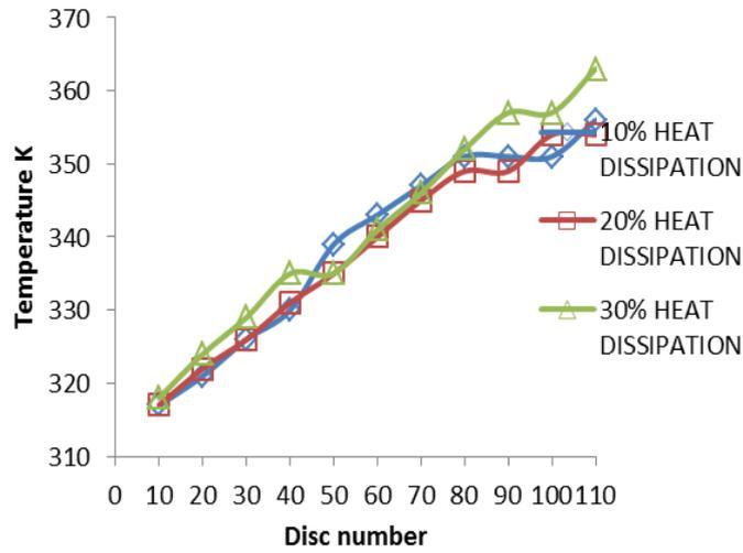
Figure 11 High voltage winding temperature
