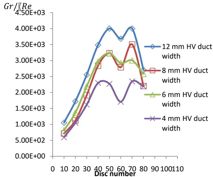
**Figure 19** High voltage winding Richardson number
