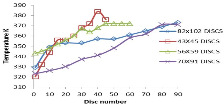
**Figure 8** Low voltage winding temperature.
