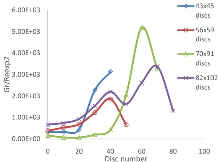
Figure 10 High voltage winding Richardson number
