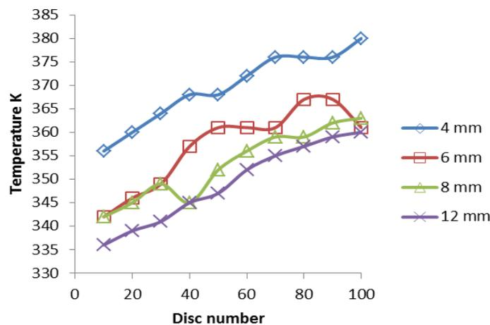
Figure 17 Low voltage winding temperature
