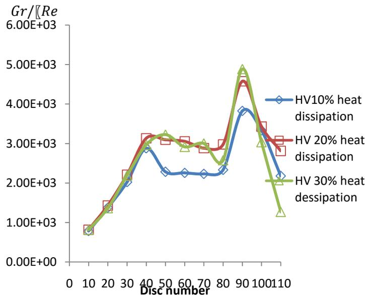
Figure 15 High Voltage winding Richardson number
