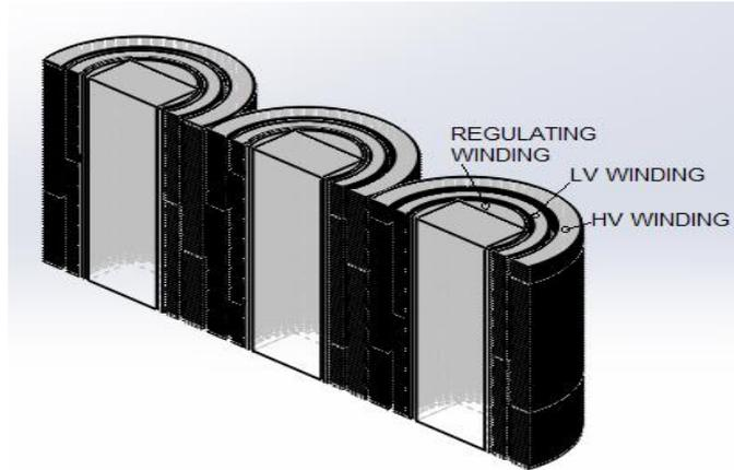
Figure 2 Internal windings of the transformer
