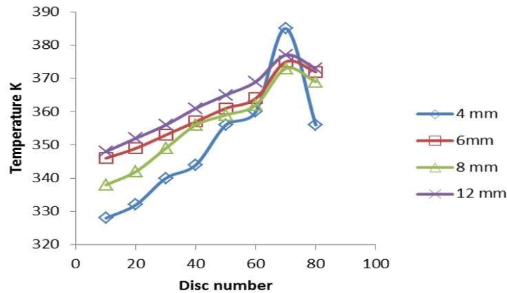
Figure 16 High voltage winding temperature
