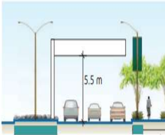
Figure 6.8 Primary Vehicle Direction Sign in the Median or Edge Zone
