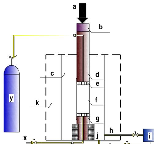
**Fig.1** Schematic of fluid-solid coupling permeability experimental system. (a) axial loading system; (b) stress sensor; (c) triaxial cell; (d) upper pressure head; (e) breathable version; (f) coal sample; (g) under pressure head; (h) the oil inlet; (i) Hydraulic pump station; (j) The oil outlet; (k) Constant temperature water bath; (x) the gas outlet; (y) High pressure gas cylinders.
