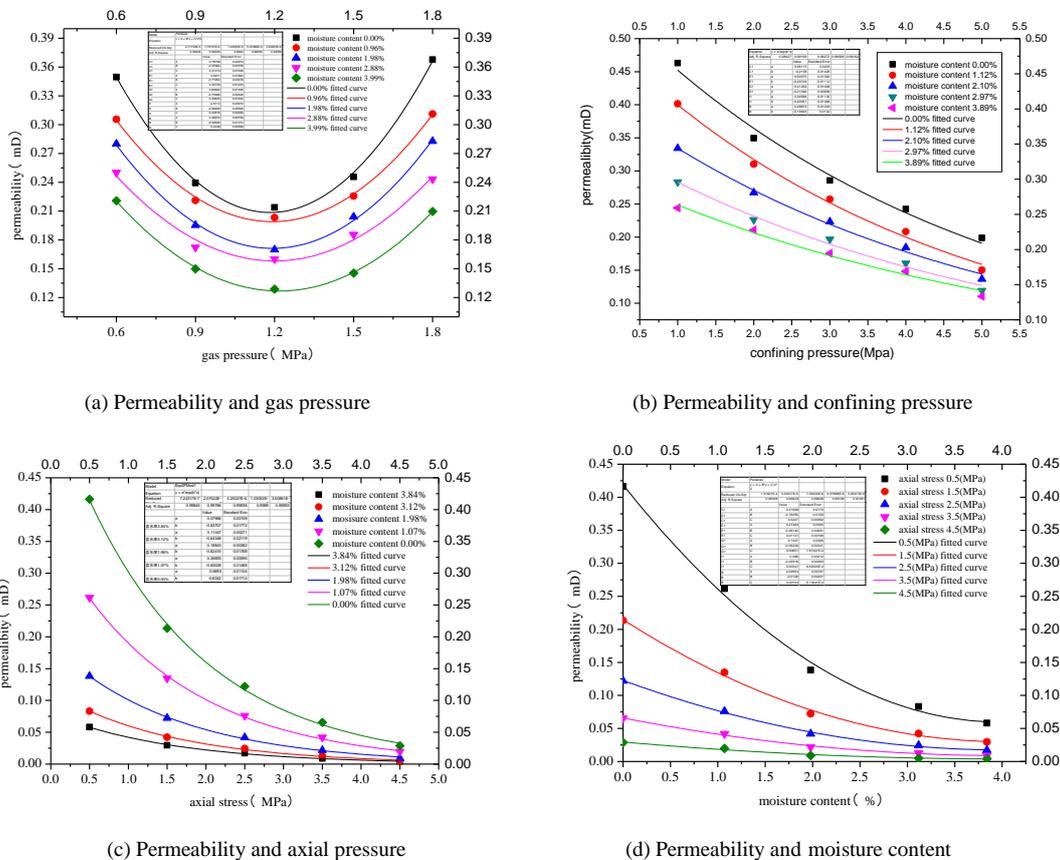
Fig. 2 The function relationship between permeability and each influencing factor
