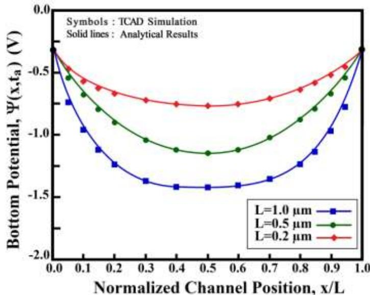
Fig. 2 The profile of bottom channel potential versus the position along the channel for various gate lengths.
