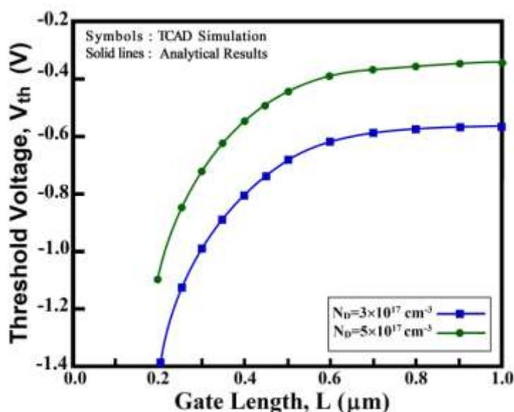
Fig. 7 The profile of threshold voltage versus the gate length for different channel concentration.
