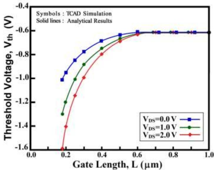
Fig. 5 The profile of threshold voltage versus the gate length for various drain biases.
