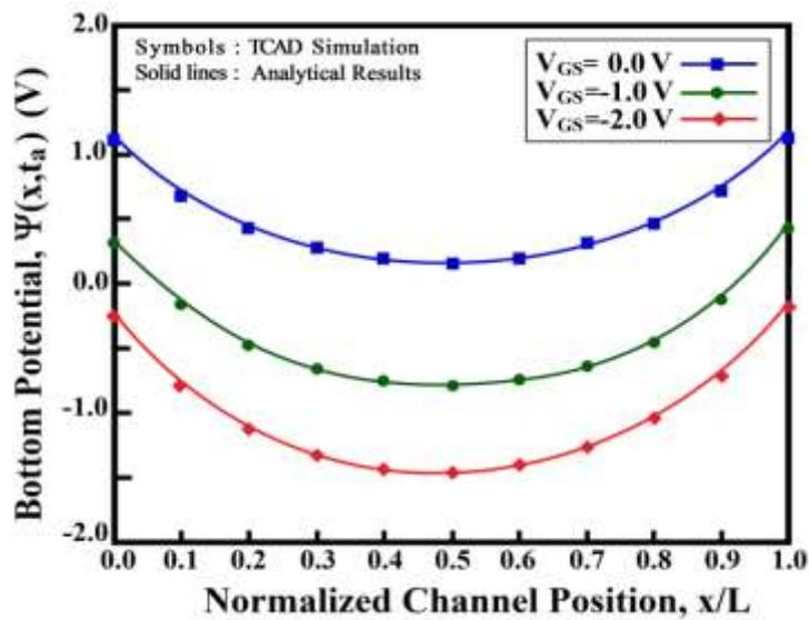
Fig. 4 The profile of bottom channel potential versus the position along the channel for various gate biases.
