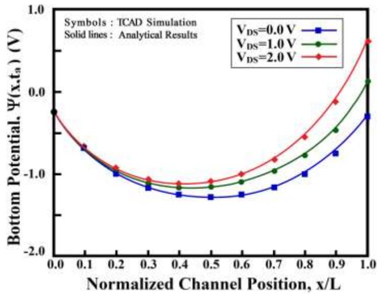
Fig. 3 The profile of bottom channel potential versus the position along the channel for various drain biases.
