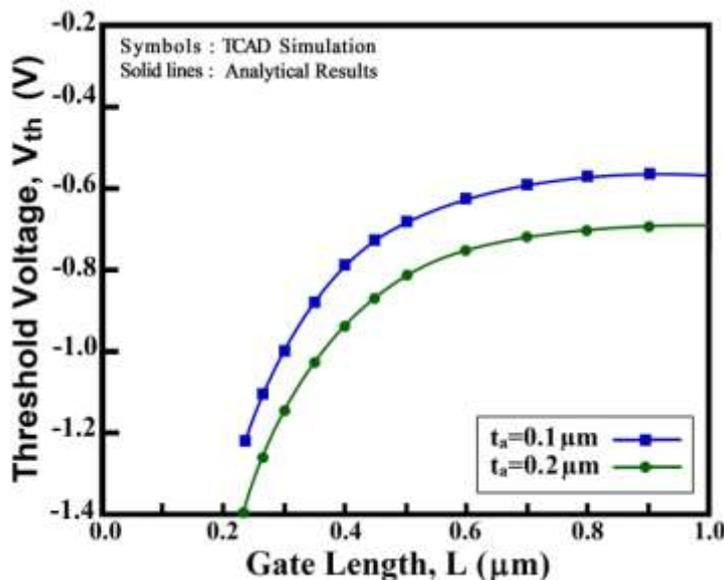
Fig. 6 The profile of threshold voltage versus the gate length for different thickness of active area.
