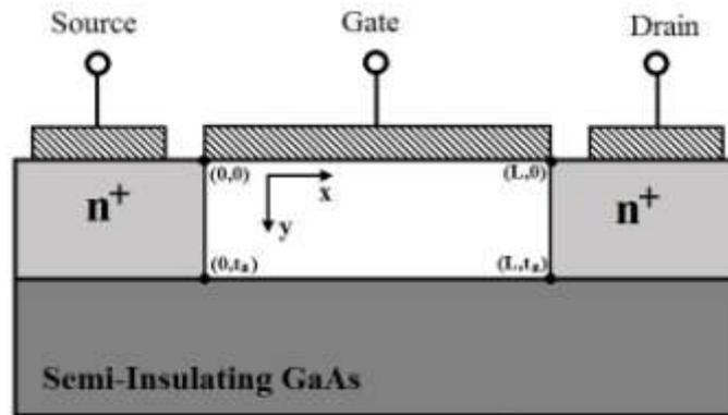
Fig. 1. The schematic view for GaAs MESFET structure
