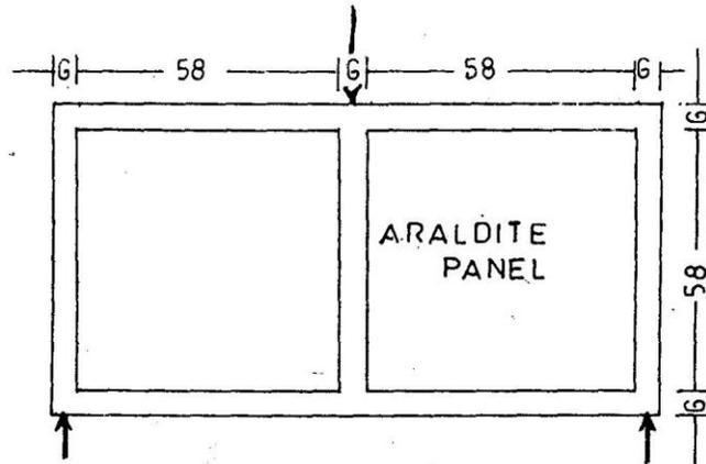
Fig.1a Testing arrangement (Dimension in mm)
