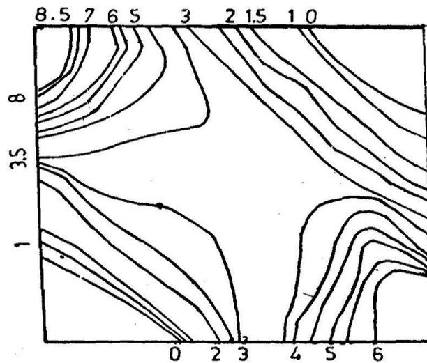
Fig 3 Principal compressive stress contours in the infill (stresses in MPa)
