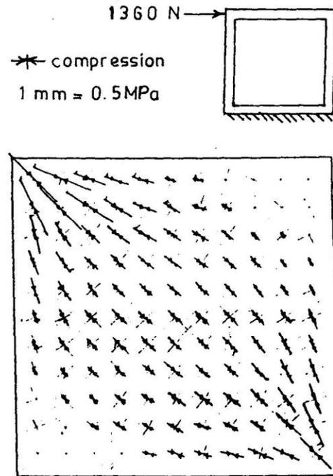
Fig 2 Flow of stresses in the panel of solid in-filled frame.
