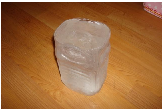
Figure 2: Ice specimen used to monitor melt rate.
