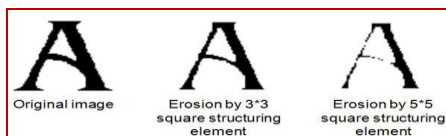
Fig 1: Example of erosion.
