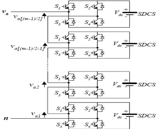
Fig.5. Single-phase structure of a m level multilevel cascaded H bridge inverter.
