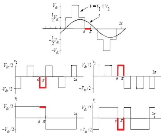
Fig.9. Capacitor voltage regulation process.
