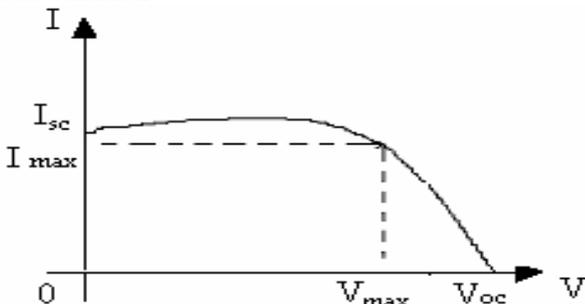
Fig. 2: Output Characteristics Of Solar Cell
