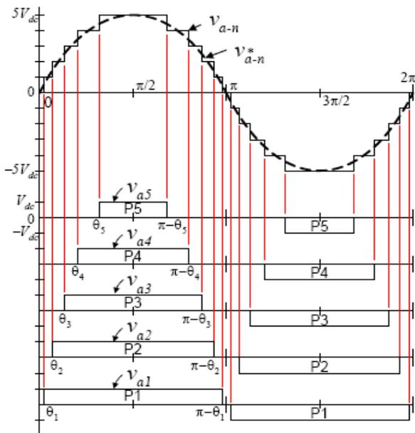
Fig.6 Output phase voltage waveform of an 11-level cascade inverter with 5 separate dc sources
