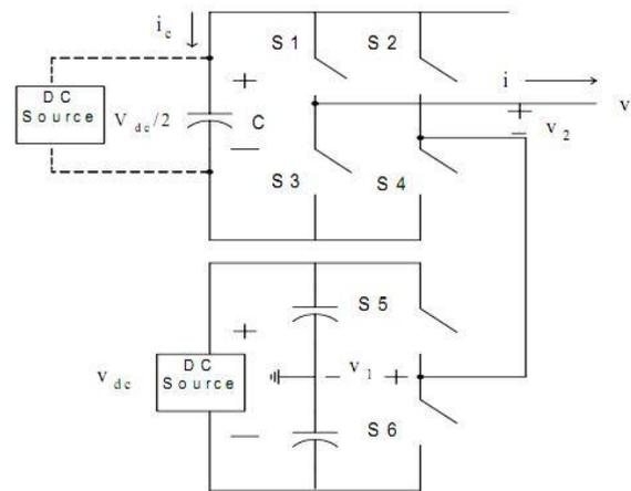
Fig.8. Simplified single-phase topology of the hybrid multilevel inverter.
