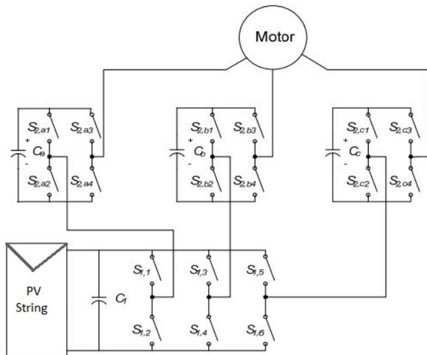
Fig.11 proposed circuit with PV array
