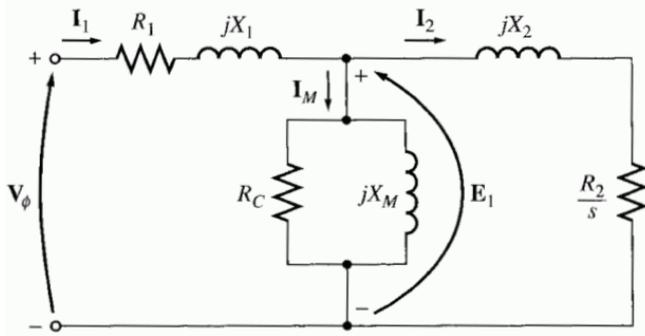
Fig.10 (b). Equivalent circuit refer to stator
