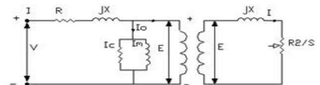
Fig. 10 (a). Steady state Equivalent circuit of an induction motor
