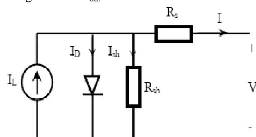
Fig. 1: Circuit model of PV solar cell
