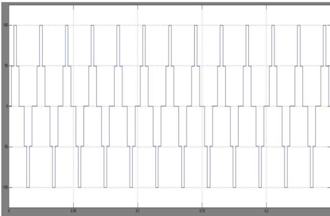
Fig.13 Five Level Inverter output Voltage with a single DC source.
