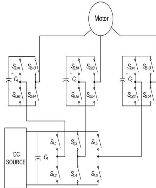
Fig.7. Topology of the hybrid multilevel inverter.
