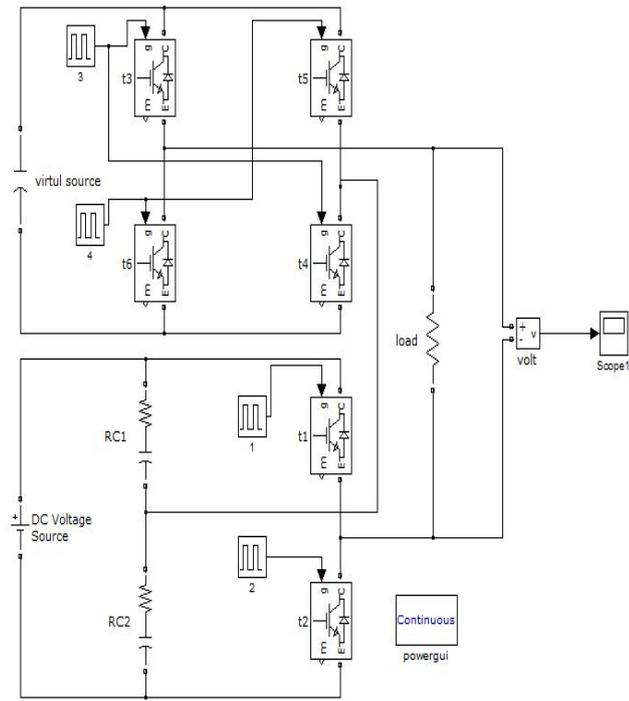
Fig.12 single phase five level inverter with a single DC source
