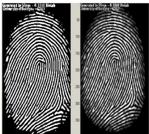
Figure 4 the Fingerprint image after adaptive binarization, Binarized image(left), Enhanced gray image(right)
